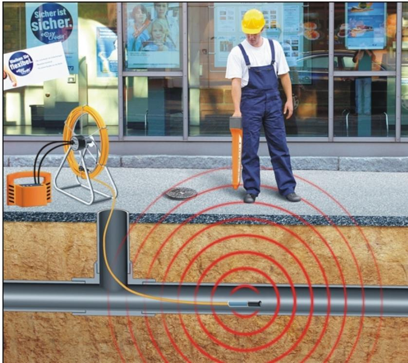
Fig. 9: Signal coupling in non-metallic pipes
