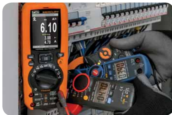
AC+DC current measurement comparison: 3.9A with RMS clamp, 4.7A with TRMS clamp, 6.1A with AC+DC TRMS clamp.
