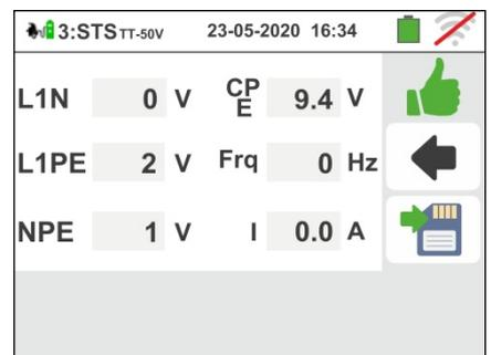
44 If the test fails, the screen like the one on the side is shown on the display. The incorrect value of the parameter is shown in red and the symbol indicates the non-ok result of the measurement.
