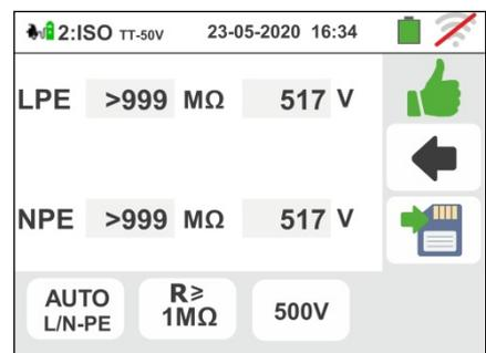
13 For three-phase EVSE systems, the measurement result of the **first L1PE test** is shown in the screen to the side. The values of the real test voltages are shown on the display
