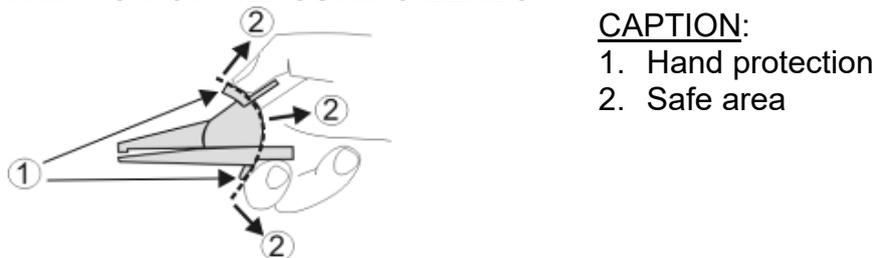
Fig. 4: Description of measuring leads
