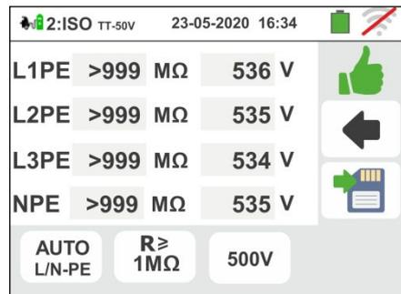
Press the **SAVE** key or touch the icon for the partial saving of the test and continue with the next test (point 20)
