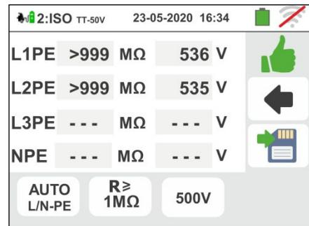
Press the **SAVE** key or touch the icon for the partial saving of the test and continue with the next test on L3 phase. The followed screen is shown on the display
