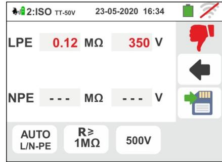
Press the **SAVE** key or touch the icon
