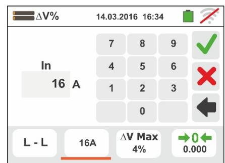
5. Touch the icon
