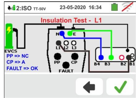
11 The test is performed by the instrument only in AUTO L/N-PE mode. Refer to § 6.2.2 for the description on setting of test parameters
