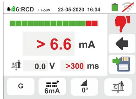
Press the **SAVE** key or touch the icon
