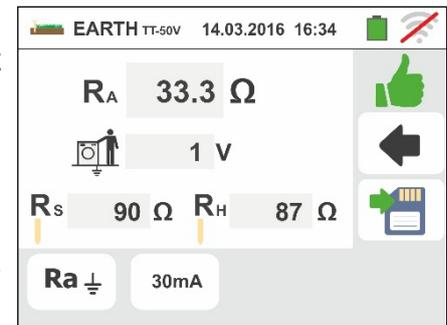
7. For **earth resistance measurement in TT systems**, in case of **negative** result (see § 13.7), the screen to the side is displayed by the instrument. It contains the value of contact voltage in the secondary display, the value of contact resistance of the voltage probe ( $R_s$ ) and the value of contact resistance of the current probe ( $R_h$ ).
