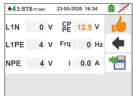
40 If the test fails, the screen like the one on the side is shown on the display. The incorrect value of the parameter is shown in red and the symbol indicates the non-ok result of the measurement.
