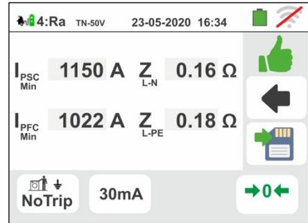
Press the **SAVE** key or touch the icon
