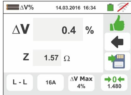
Press the **SAVE** button or touch the
