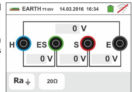
5. Touch the
