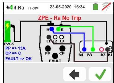
47 The test is performed by the instrument **only in "NoTrip" mode**. Refer to § 6.4.12 for the description on the setting of the test parameters relative to the trip out current of the RCD, **absence of neutral conductor (only possible measurement)** and the preliminary calibration of the measuring terminals
