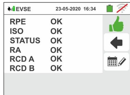
4. Touch the
