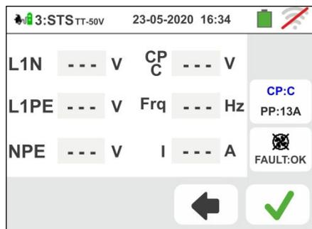
31 The result of the measurement is shown in the screen to the side. The symbol indicates the correct result of the measurement. The symbol also indicates a positive result of the measurement but with values outside the limits present in the Table 4.
