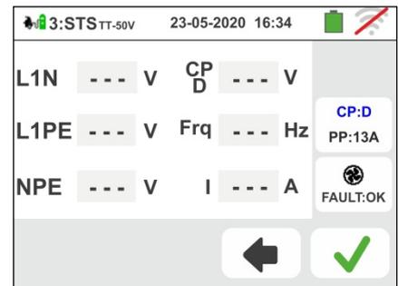
35 The result of the measurement is shown in the screen
