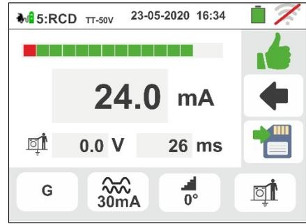
Press the **SAVE** key or touch the icon
