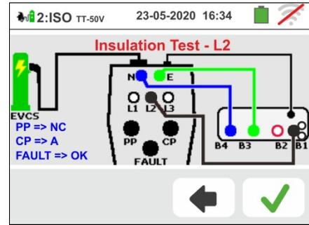
15 The measurement result of the **L2PE test** is shown in the screen to the side. The values of the real test voltages are shown on the display
