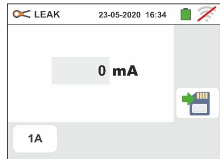
2. Touch the
