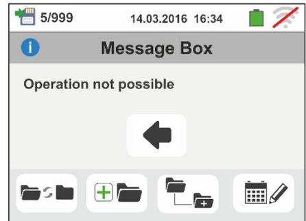
3. In case tries to create a sub-node by using a just used name, the instrument provides the warning screen shown to the side and is necessary to define a new name
