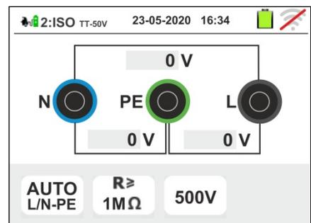
12 For single-phase EVSE systems, the measurement result is shown in the screen to the side. The values of the real test voltages are shown on the display. The symbol indicates the correct result of the measurement.
