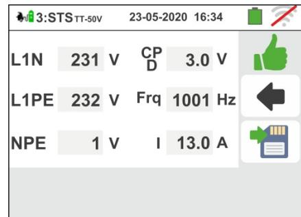
36 If the test fails, the screen like the one on the side is shown on the display. The incorrect value of the parameter is shown in red and the symbol indicates the non-ok result of the measurement.
