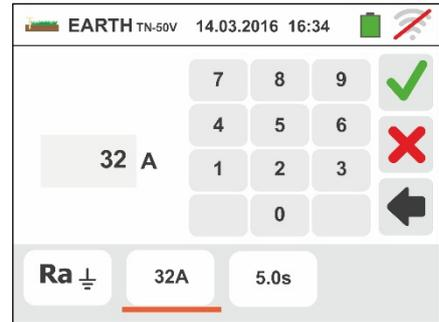
6. Touch the
