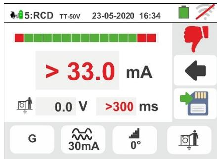
Press the **SAVE** key or touch the icon
