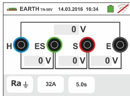
5. Touch the
