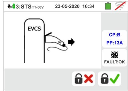
Press the icon
