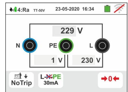
48 During this whole phase, do not disconnect the measuring terminals of the instrument from the system on test. In case of positive outcome (global earth resistance lower than the ratio between the limit contact voltage and the RCD tripping current - see § 13.8), the screen to the side is shown by the instrument in which the contact voltage value is indicated on the secondary display.
