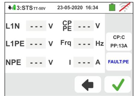
39 The result of the measurement is shown in the screen
