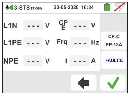
43 The result of the measurement is shown in the screen to the side. The symbol indicates the correct result of the measurement. The symbol also indicates a positive result of the measurement but with values outside the limits present in the Table 4
