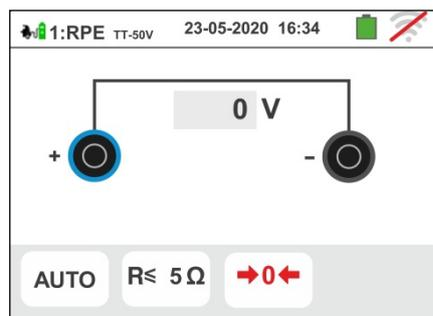
7. The value of the result is shown in the upper part of the screen while the partial values of the tests with inverted polarity of the test source in addition to the actual test currents are shown in the fields "R +" and "R-"
