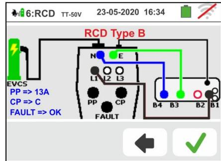
64 The test is performed by the instrument considering **only General RCD of STD (G) type, type B/B+ and in Ramp mode (
