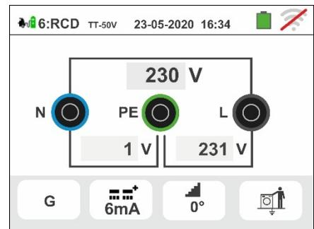
65 Move the third slide bar reference by selecting the desired rated current of the differential switch between the options: **6,10, 30, 100, 300mA**
