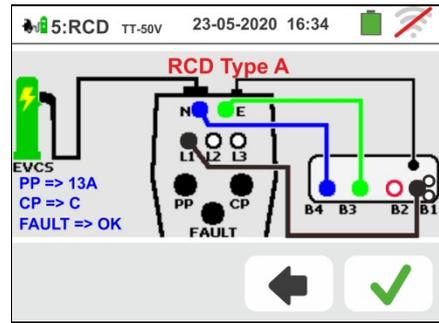
56 The test is performed by the instrument considering **only General RCD of STD (G) type, type A/F and in Ramp mode (
