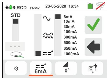
66 **Ramp mode
