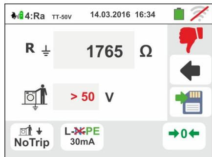
Press the **SAVE** key or touch the icon
