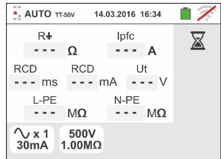
8. In case of **positive** result of the three test sequentially performed as **NoTrip** (see § 13.8), **RCDX1** (see § 13.4) and **MΩ L/N-PE** the symbol is shown and the screen to the side is displayed by the instrument
