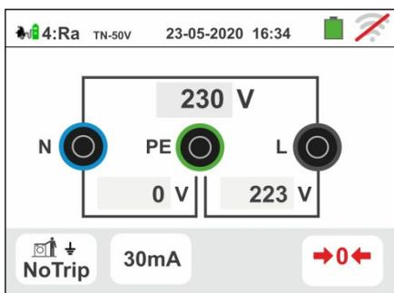
52 During this whole phase, do not disconnect the measuring terminals of the instrument from the system. In case of positive result (**Z<sub>L-PE</sub> or Z<sub>L-N</sub> LOWER or EQUAL to limit impedance relative to protection device within the specified time** – see § 13.7), the screen to the side is displayed by the instrument. Press again the **GO/STOP** key for a few seconds to repeat the test
