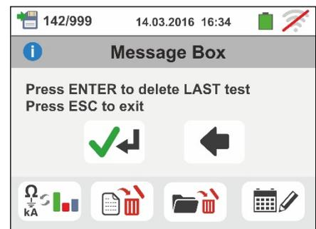
5. Touch the
