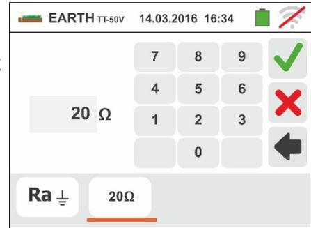
6. Press the **GO/STOP** key. During this whole stage, do not disconnect the measuring leads of the instrument from the system under test. The
