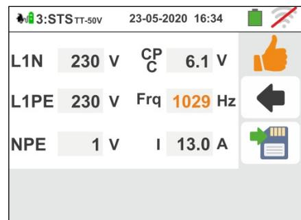
32 If the test fails, the screen like the one on the side is shown on the display. The incorrect value of the parameter is shown in red and the symbol indicates the non-ok result of the measurement.
