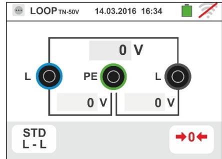
2. Move the left slide bar reference by selecting the icon to execute the measurement with the accessory IMP57.
