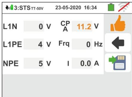
22 If the test fails, the screen like the one on the side is shown on the display. The incorrect value of the parameter is shown in red and the symbol
