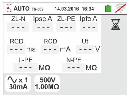
8. In case of **positive** result of the three test sequentially performed as **NoTrip** (ZL-N and ZL-PE<199Ω), **RCDX1** (see § 13.4) and **MΩ L/N-PE** the symbol is shown and the screen to the side is displayed by the instrument
