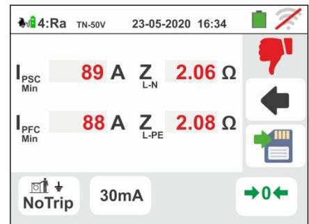
Press the **SAVE** key or touch the icon
