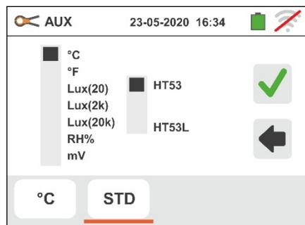
3. **If the HT53L probe is used**, select the color of the LED source under test from the options: **STD (standard white light source), White, Red, Yellow, Green, Blue** and **Purple** as shown in the screen to the side
