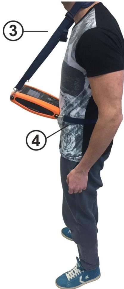
Fig. 43: Complete mounting of set strap
