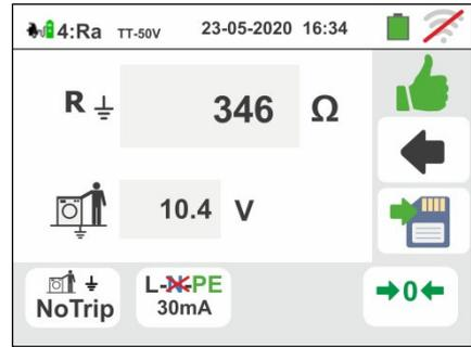
Press the **SAVE** key or touch the icon
