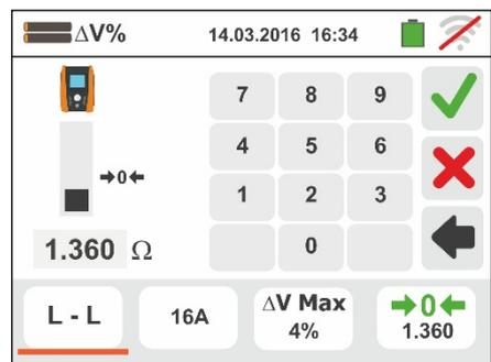
4. Touch the icon
