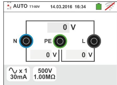
2. Move the left slide bar reference by selecting the waveform of the differential switch between the options:  $\text{⏏}$  (type AC),  $\text{⏏}$  (type A/F),  $\text{⏏}$  (type B/B+). Move the second slide bar reference by selecting the desired rated current of the differential switch between the options: **6mA, 10mA, 30mA, 100mA, 300mA** Move the third slide bar reference by selecting the type of the test between the following options:
