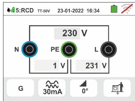
57 Move the third slide bar reference by selecting the desired rated current of the differential switch between the options: **6,10, 30, 100, 300, 500, 650mA**
