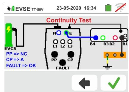
6. The RPE test is performed by the instrument **only in AUTO mode**. Set the limit threshold value and calibrate the measurement cables as shown in § 6.1
