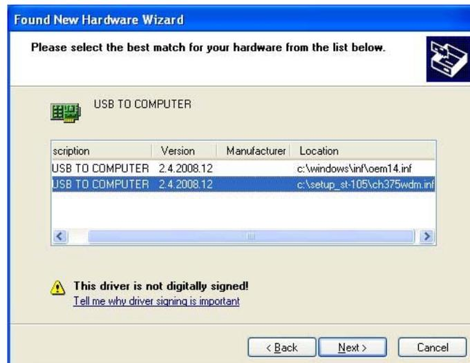
7. The installation procedure of the driver is started by the PC
