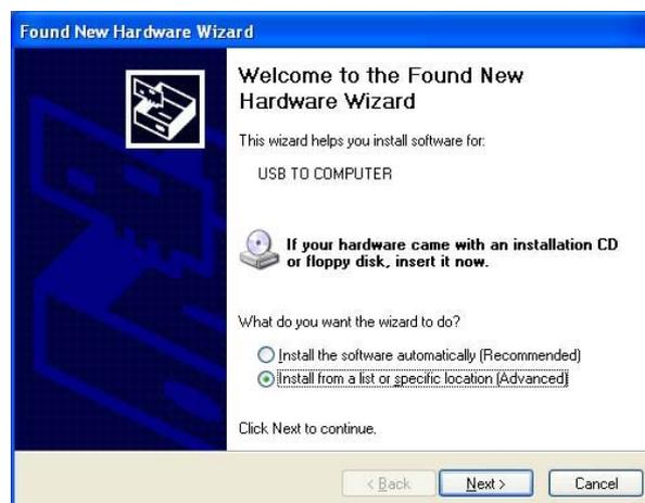
4. Select the option "Install from list or specific location" in order to select the driver from a specific folder and click on the "Next" key. The PC shows the following screen:
